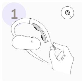
Insert the tip of the sensor removal tool into the small round opening at the end of the ear hook. Then, push up gently until you hear a click.
